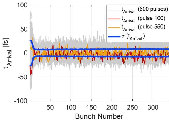
Figure 3: Mean free arrival time of BAM2. The grey lines show the arrival time of 600 pulses and the blue solid line the standard deviation  $\sigma(t_{\text{Arrival}})$ . The intra-train beam-based feedback at ACC1 runs together with BACCA.
