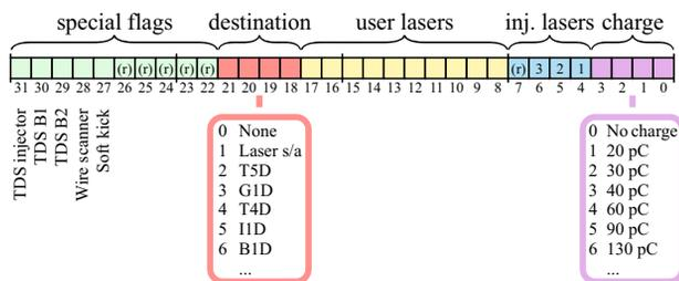
Figure 3: The 32-bit timing word encodes the destination and the maximum charge for a bunch as well as information for various subsystems.
