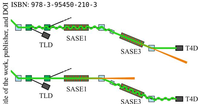
Figure 2: Illustration of the fresh bunch technique. *Top*: Bunches destined for lasing in SASE3 are deflected by one of the TLD kickers so that they oscillate through SASE1; afterwards, an orbit correction brings them onto a straight trajectory through SASE3. *Bottom*: Bunches destined for lasing in SASE1 receive no kick and therefore follow a straight trajectory in SASE1 and oscillate through SASE3.
