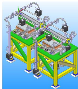
Figure 1: Technical drawing of the supports for the two PolariX TDSs at FLASH2. Courtesy of M. Föse.
