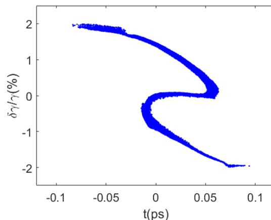
Figure 2: Electron distribution of the compressed beam in longitudinal phase space at linac system exit. Residual beam energy chirp is compensated by a 1 m corrugated pipe dechirper.
