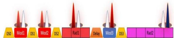
Figure 1: The layout of the two-stage cascaded scheme.
