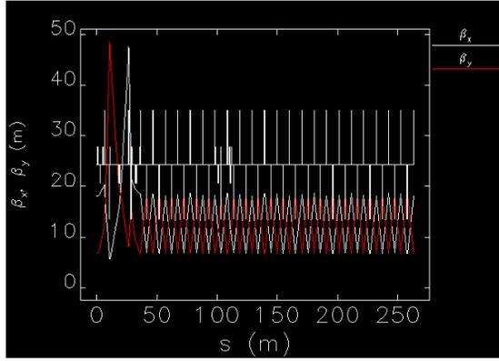
Figure 3: The lattice of two-stage cascaded EEHG/HGHG scheme.
