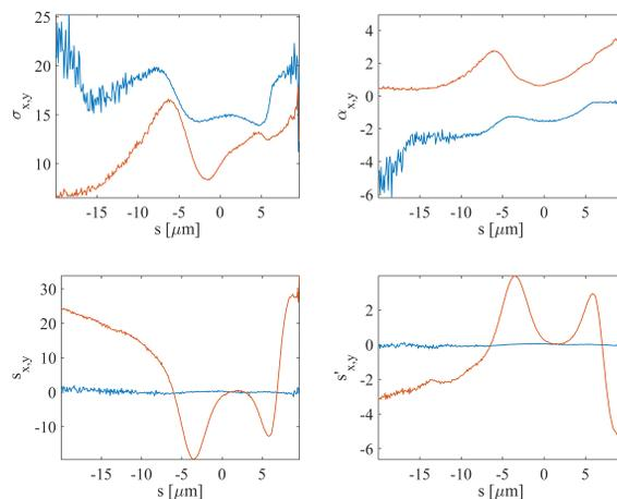
Figure 5: Twiss parameters of  $x$  (blue) and  $y$  (red) of the electron beam: Top-left: the sliced beam size. Top-right: the sliced  $\alpha_{x,y}$ . Bottom-left: the sliced transverse offsets. Bottom-right: the angular deviation. Beam tail is at the left side of  $s$  coordinate axis.
