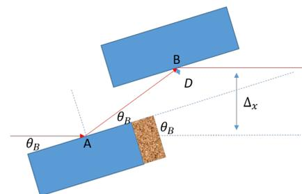
Figure 2: Reflection monochromator with double-crystal for self-seeding.
