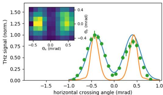
Figure 4: Normalized THz signal (dots) under variation of the horizontal crossing angle at zero vertical angle together with SPECTRA calculations without (orange) and including (blue) the laser divergence (see Fig. 3). Inset: THz signal under coarse variation of the horizontal and vertical crossing angles  $\theta_{x,y}$  [4].
