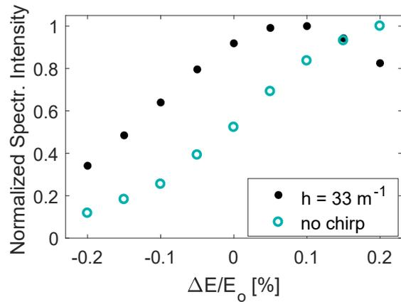
Figure 6: Impact of energy jitter on the peak intensity of the output spectrum for a chirped and an unchirped electron beam. We assume that for  $\Delta E/E_0 = 0$  the energy is the nominal one. The intensity is normalized to the maximum one for each chirp.
