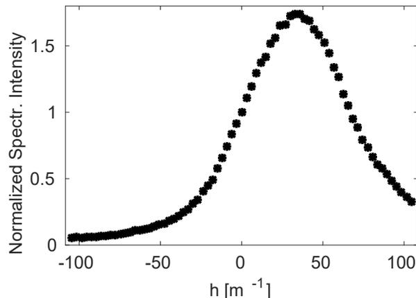
Figure 3: Impact of the electron beam energy chirp on the peak spectral intensity of the output spectrum. The intensity is normalized to the one of the unchirped electron beam. The  $h = 0 \text{ m}^{-1}$  is defined with the resonance condition.
