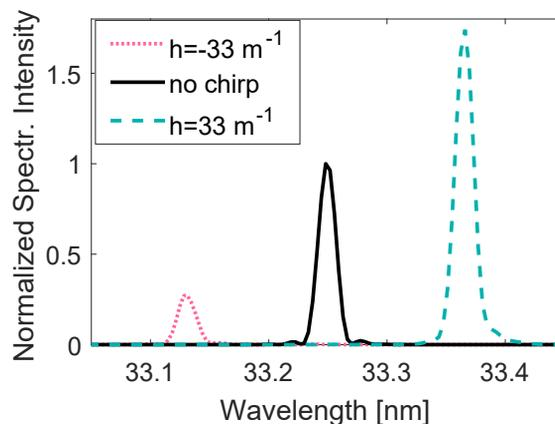
Figure 4: Impact of an initial electron beam energy chirp on the output spectrum in comparison with the spectrum generated with an unchirped electron beam. The intensity is normalized to the one of the unchirped electron beam.
