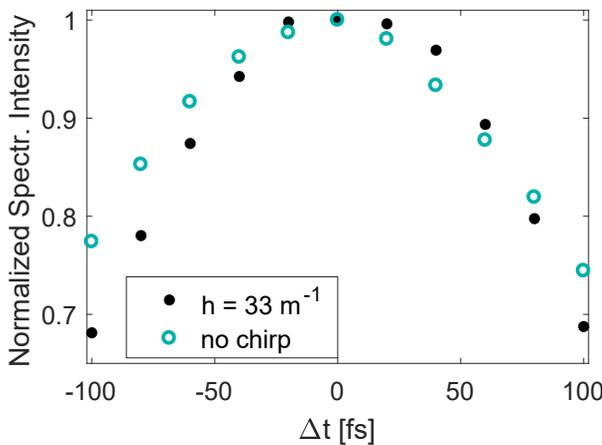
Figure 5: Impact of timing jitter on the intensity of the output spectrum for a chirped and an unchirped electron beam. We assume that for  $\Delta t = 0$  the peak current of the electron beam overlaps with the peak power of the seed laser in the middle of the modulator. The intensity is normalized the maximum intensity for each chirp.
