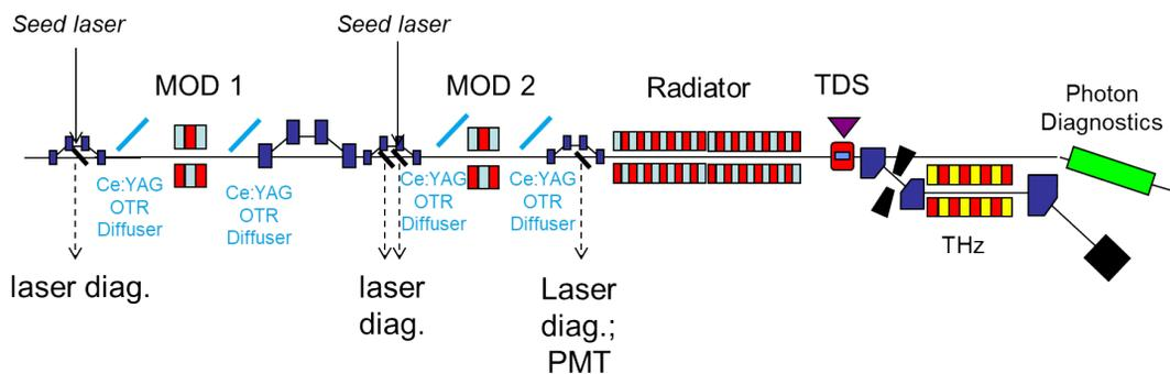
Figure 1: Proposed FLASH1 seeding beamline and fundamental diagnostics.
