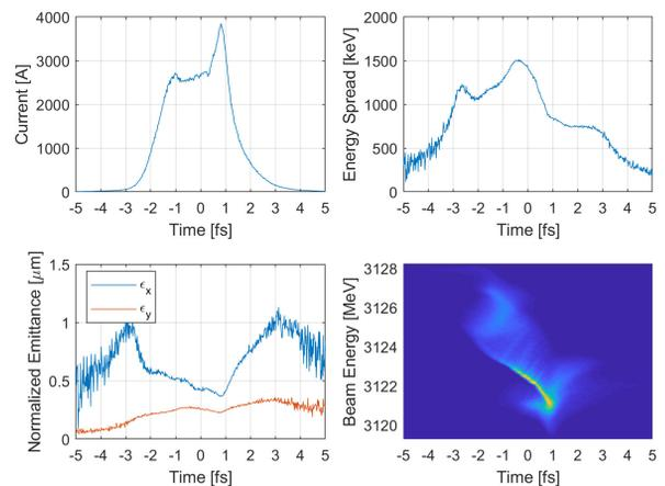
Figure 4: Electron beam slice parameters and longitudinal phase space at the linac exit (after BC2) for 10 pC charge. Bunch head is to the left.
