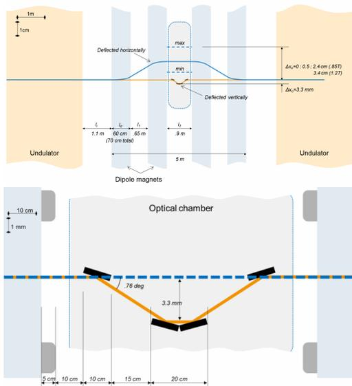
Figure 3: Concept of chicane and optical delay line.
