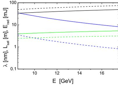
Figure 2: Radiation wavelength (blue), saturation length (black), and radiation pulse energy in the saturation (green) versus electron energy. Solid lines and dashed lines correspond to closed and open undulator gap, respectively. Undulator period is equal to 11 cm. Bunch charge is 250 pC [6]. Simulations are performed with code FAST [7].
