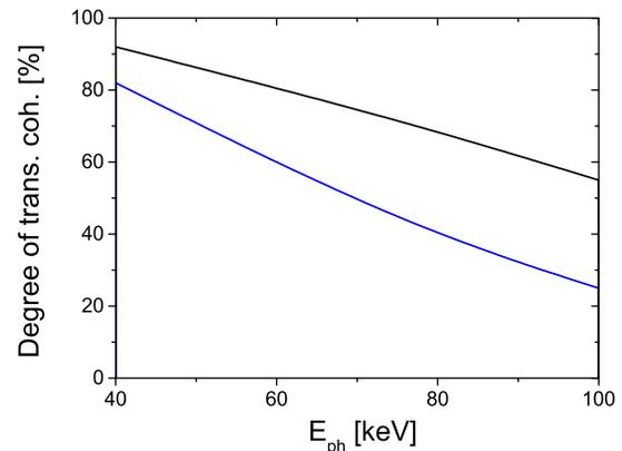
Figure 4: Expected degree of transverse coherence (see the definition in [17]) of SASE FEL radiation as a function of photon energy. Blue line: normalized emittance is  $0.3 \text{ mm mrad}$ . Black line: normalized emittance is  $0.2 \text{ mm mrad}$ . Electron beam energy is 17.5 GeV. Estimates were done using the results of Ref. [17].
