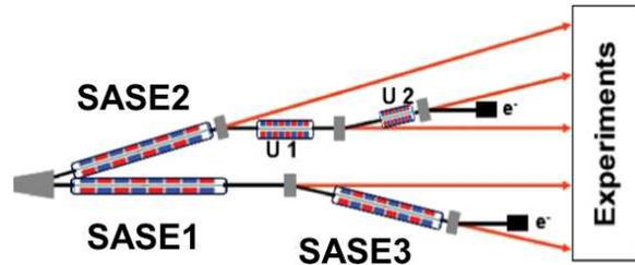
Figure 1: Layout of undulator tunnels of the European XFEL
