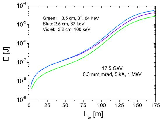
Figure 3: FEL pulse energies versus undulator length for the three undulator cases: superconducting (blue), in-vacuum (violet), and standard out-of-vacuum with the 3<sup>rd</sup> harmonic lasing (green).
