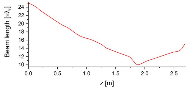
Figure 2: The full electron bunch length in units of resonant wavelength. The initial energy chirp at  $z = 0$  m is seen to cause the electron pulse to compress and then will decompress longitudinally.
