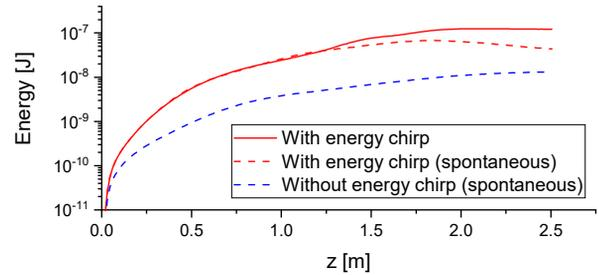
Figure 3: Radiation energy as a function of distance  $z$  through the undulator. Two of the plots (red) are for the chirped pulse including (solid) the FEL interaction and (dashed) without the FEL interaction. The case without energy chirp or FEL interaction (blue dashed) gives an energy growth with a quasi-linear dependence with  $z$ , corresponding to shot-noise spontaneous emission without significant CSE contribution.
