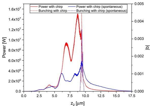
Figure 5: The radiation power profile (solid red) and the electron bunching parameter (dashed red) as a function of  $z_2 = (ct - z)$  at  $z = z_{sat} = 1.95$  m through the undulator for the energy chirped case and corresponding case for the FEL interaction ‘switched off’ (solid blue and dashed blue).
