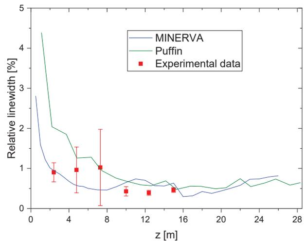
Figure 3: Comparison of the measured relative linewidth in red (data courtesy of L. Giannessi) with that found in the simulations (blue for MINERVA and green for PUFFIN).
