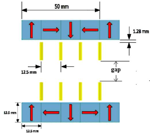
Figure 1: Schematic of one Period of harmonic Undulator( $l=3$ ).
