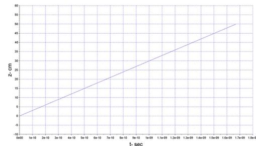
Figure 2: Trajectory of electron along 'x' and 'z' in Planar undulator (Numerical calculation).
