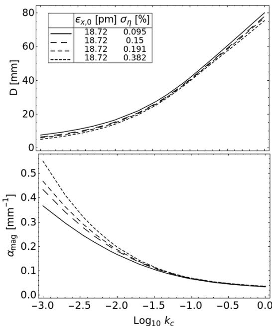
Figure 4: Optimal dispersion (top) and magnetic gradient (bottom) vs  $k_c$  for varying  $\sigma_\eta$ .
