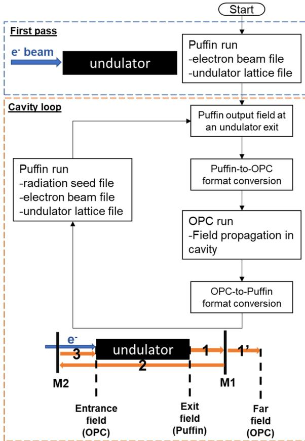
Figure 3: The diagram shows the flow chart of the RAFEL simulation, including the first pass, conversion script, and the cavity loop which is a simple Bash shell script. (1) The first propagation using OPC from the undulator exit to mirror-1 (M1) with a hole out-coupling and the far-field diagnostic point (1'). (2) The second propagation from a reflected optical beam at M1 to mirror-2 (M2). (3) The third propagation from M2 to the undulator entrance as the next loop radiation seeding.
