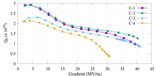
Figure 2: Vertical tests of TARLA cavities.
