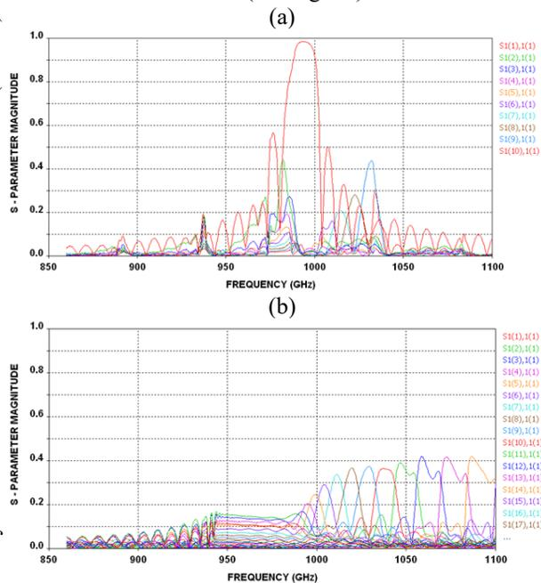
Figure 2: 3D simulations of Bragg resonators at THz-band using using *CST MICROWAVE STUDIO* software. (a) Advanced Bragg reflector, (b) conventional Bragg reflector.
