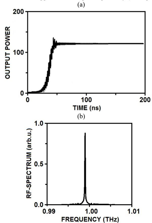
Figure 3: Results of simulations of FEL – oscillator in the frame of averaged theory. (a) Establishment of stationary narrow-band oscillation regime, (b) radiation spectrum.
