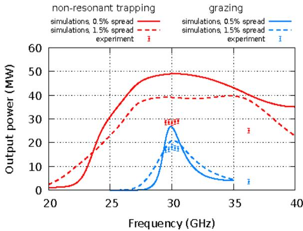
Figure 2: Simulations of the FEM-amplifier: output power versus the frequency for the non-resonant trapping regime (red lines) and grazing regime (blue lines). Experimental results (the output powers measured in the examined regimes) are shown by dots of corresponding colours.
