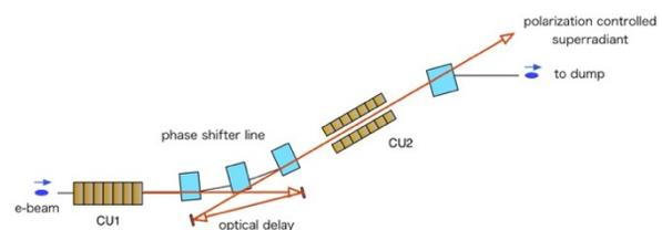
Figure 1: Crossed-undulator configuration. Path length difference between the beam and THz superradiance has to be varied in the phase shifter line. Since the e-beam transport matrix element of  $R_{56}$  should be variable for compensation of bunch lengthening due to momentum dispersion, the optical delay is controlled so as to satisfy the radiation phase difference from 0 to  $2\pi$ .
