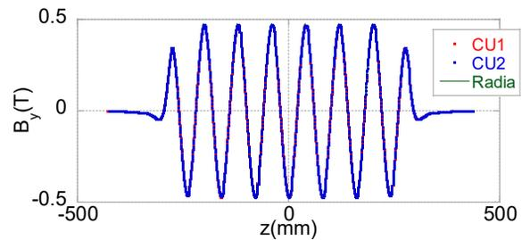
Figure 3: Measured magnetic fields in the direction perpendicular to deflecting planes of both CU1 and CU2. RADIA calculation is also plotted.
