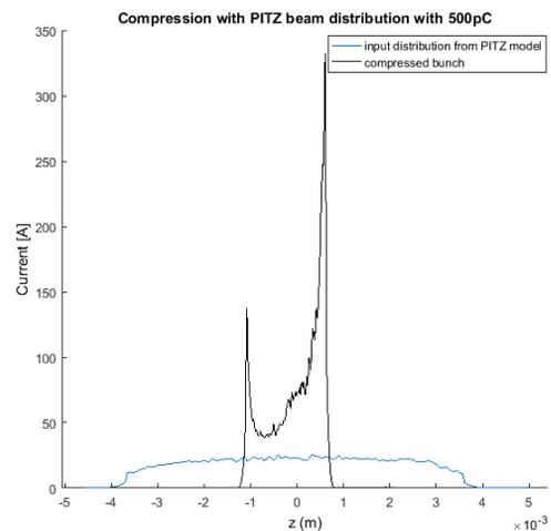
Figure 4: Simulated bunch compression of the PITZ beam distribution with 500 pC bunch charge and 17 MeV mean energy using CSRtrack code. The tail is on the left side.
