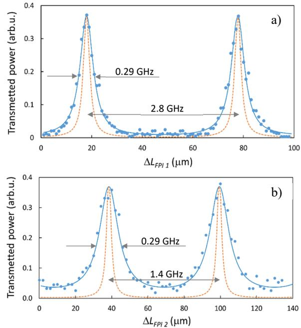
Figure 2: Fine structure of KAERI FEL radiation spectrum at central wavelength of 117  $\mu$ m (2.6 THz) measured by Fabry-Perot interferometers with lengths  $L_{FPI-1} = 53.6$  mm (a) and  $L_{FPI-2} = 107.2$  mm (b). Dots: experimental points, blue solid lines: best fitting to experimental points. Dashed orange lines: instrumental functions of interferometers.
