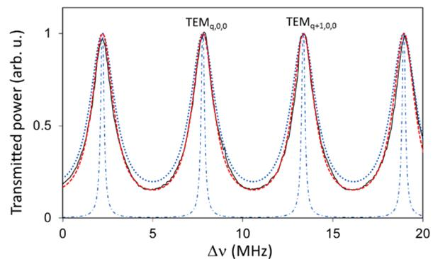
Figure 4: Hyperfine structure of THz NovoFEL radiation at central wavelength of 164  $\mu$ m (1.83 THz). Solid black line: measured NovoFEL radiation, dashed red line: instrumental function of ultra-long waveguide vacuum FPI with 30- $\mu$ m nickel meshes, blue dotted line: spectrum appreciably differing from experimental one as a result of convolution of laser line with relative spectral width of  $10^{-7}$  (blue chain line) and instrumental function.
