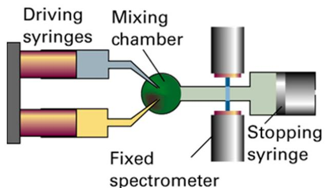
Figure 1: Geometry of the stopped flow apparatus.
