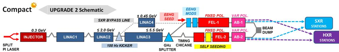
Figure 1: Schematic of CompactLight with Upgrade 2 applied.
