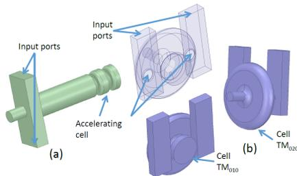
Figure 2: Proposed input couplers: (a) mode launcher type; (b) new coupler with TM<sub>020</sub> cell.
