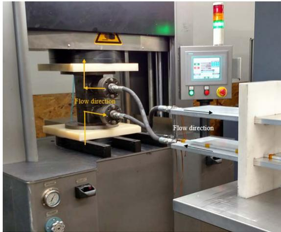
Figure 2: The right angle diverter showing flow direction.
