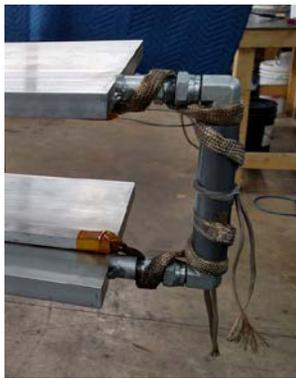
Figure 3: The return end manifold.
