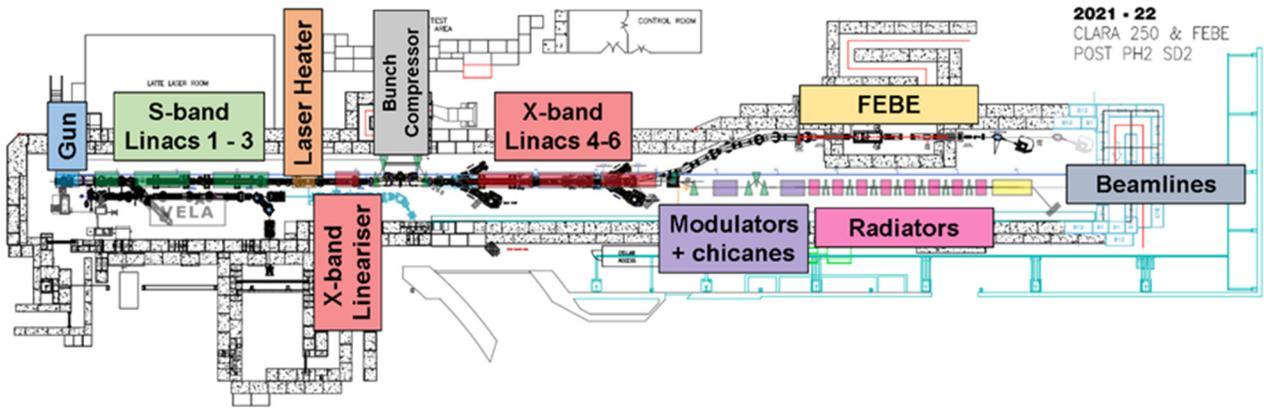
Figure 2: Layout of CLARA phase 2 showing the potential XARA layout overlaid. CLARA linac 4 (S-band) is replaced with 3-4 X-band linacs to achieve  $\sim 1$  GeV/c beam momentum. The FEL and beamlines section is indicative and could extend beyond the present building if required.
