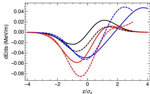
Figure 3: Wakes calculated in 1D model are shown by solid lines: black — in the middle of the second magnet ( $s = -0.75 \text{ m}$ ), blue — at the center of the chicane ( $s = 0$ ), and red — in the middle of the third magnet ( $s = 0.75 \text{ m}$ ). Dashed lines (with the corresponding color) are calculated for the same locations using a 2D version of Eq. (2). The coordinate  $z$  is normalized by the rms bunch length,  $\sigma_z(s)$ .
