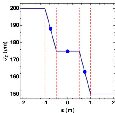
Figure 2: Variation of the bunch length  $\sigma_z(s)$  through the second and third magnets of the chicane (the magnet edges are shown by red dashed lines). The coordinate  $s = 0$  corresponds to the center of the chicane. The blue dots show three positions in the chicane where the CSR wake was calculated.
