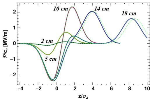
Figure 1: Longitudinal wake in the bunch as a function of distance from the entrance edge of the bend shown by a number near each curve. The longitudinal coordinate  $z$  in each case is measured from the center of the bunch.
