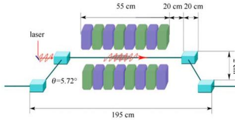
Figure 4: Layout of a typical laser heater.
