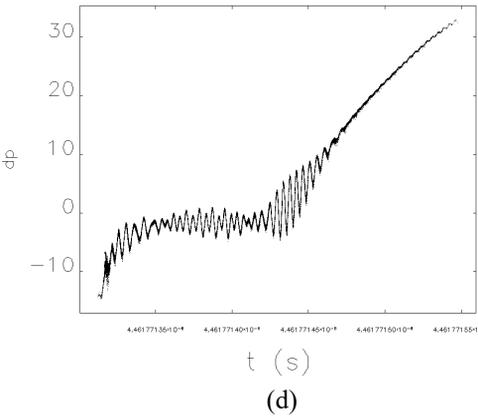
Figure 3: Longitudinal phase space of the beam at the exit of SHINE linac, with (a) 60  $\mu\text{m}$ , (b) 90  $\mu\text{m}$ , (c) 120  $\mu\text{m}$ , (d) 150  $\mu\text{m}$  initial density modulation.
