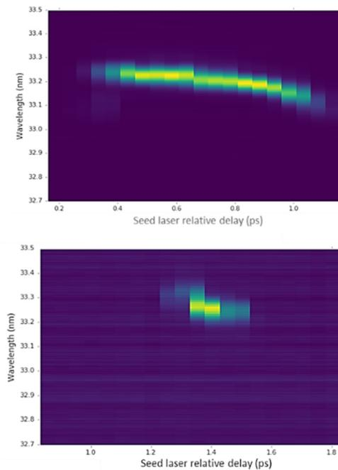
Figure 4: Spectrum of the first stage of FERMI HGHG FEL2 vs. seed laser delay. The seed laser is superimposed to the whole electron beam (top), and to a single beamlet produced with scraping in BC1 (bottom). The spectrum intensity is normalized in both plots to the peak value. The seed is time-shifted in steps of 50 fs, 20 shots are consecutively recorded for each delay value.
