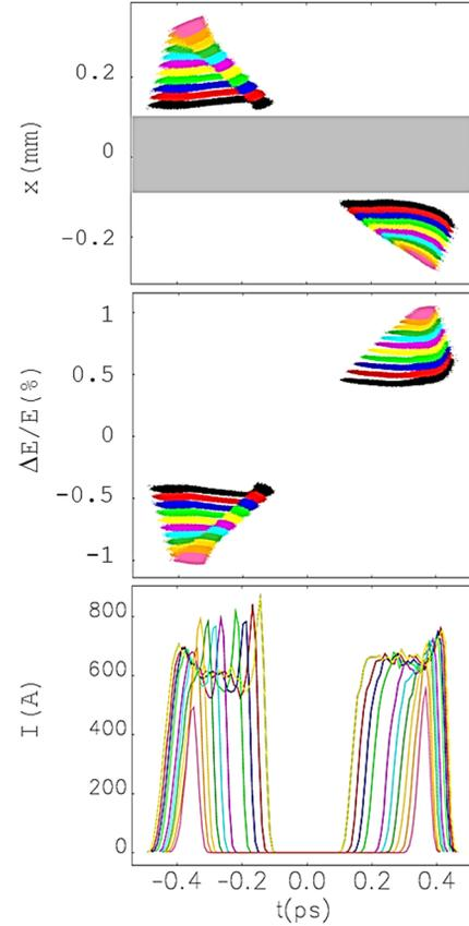
Figure 2: From top to bottom, longitudinal phase space, top view (with shadow of the 2 mm septum thickness) and current profile of the two beamlets at the undulator entrance, for a mask slit width in the range 3–8 mm, and apertures width of 1–6 mm. Bunch head is on the left. The linac RF phases were optimized for one beamlet's duration only (black).
