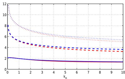
Figure 1: Quadrupole QI. The number of correct decimal digits in the approximation of the transport matrices  $M^\pm(k_0)$  by conventional rectangular model (solid curves), and by zeroth (dashed curves) and first (dotted curves) order Steffen models. Red and blue colors refer to the focusing and defocusing matrices, respectively.
