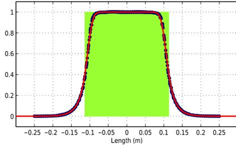
Figure 2: Quadrupole QI. Red curve shows its gradient shape function  $k(s)$ , which was obtained (in the form of some combination of the Enge functions) as a fit to the measured data represented in this figure by the blue dots. Green rectangle shows effective field boundary  $l_e$ .
