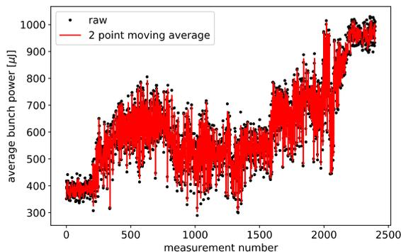
Figure 3: Extremum Seeking simultaneous optimization of 16 phase-shifters gaps [9].
