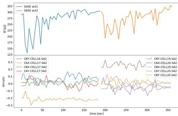
Figure 6: Sequence of optimization with aircoils in SA-SE2 undulator.
