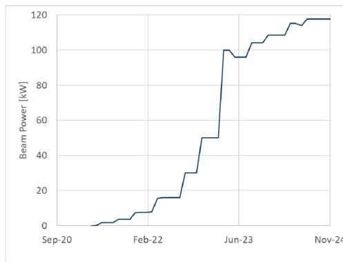
Figure 7: Ramp up of beam power during machine start and early years of operation.
