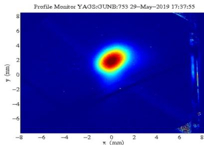
Figure 3: Profile of first LCLS-II electron beam.
