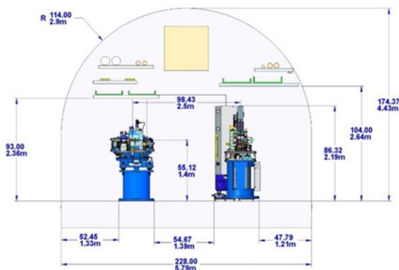
Figure 5: Arrangement of HXR (left) and SXR (right) undulators in the FEL tunnel.
