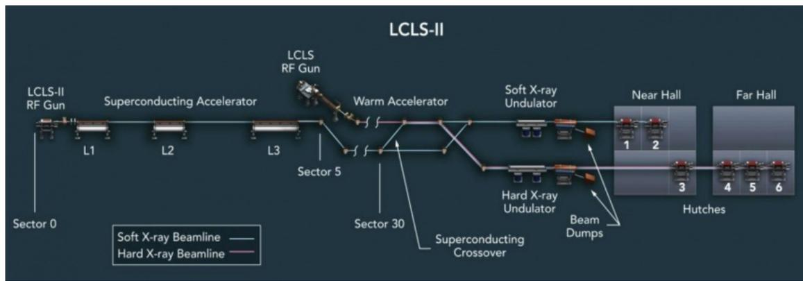
Figure 1: Schematic layout of the LCLS-II Facility.
