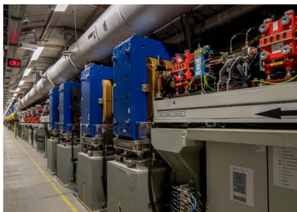
Figure 3: First bunch compression chicane.
