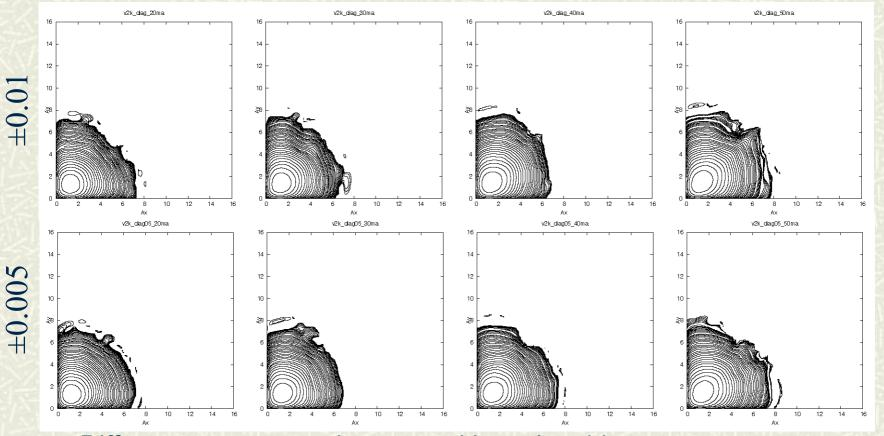
Different tune separation caused by solenoids
