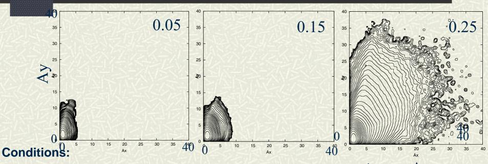
arc tunes separation  $A_{202}$  by the doublet (D3,F3) & F1 lenses, beta<sup>\*</sup>x,y kept equal; circular modes and a wider tune split produced by twist 0.79kGs\*66.5524cm: Qx = 4.1115, Qy=2.0893,
