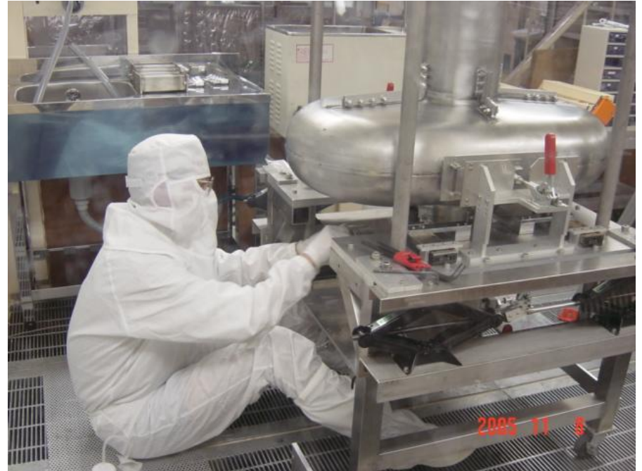
Set Flanges of Beam Pipes and Ports in Class 100 Clean
