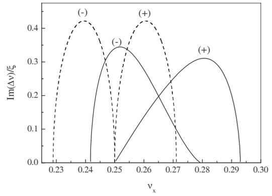
Figure 4: The stopbands of coherent oscillations near the resonance  $1/4$ . Solid line – Landau damped coherent oscillations, dashed line – monochromatic bunches, the symbols  $(\pm)$  mark the curves for modes  $(\pm)$ ,  $\xi = 0.05$ .
