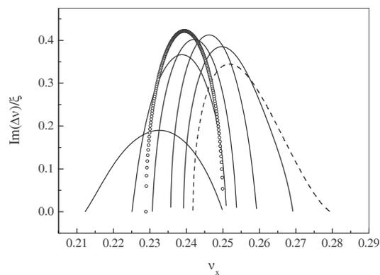
Figure 6: Modifications of the stopband of the  $(-)$  mode near  $\nu_x = 1/4$  due to octupoles. Solid lines right to left  $a/\xi = 0.1, 0.2, 0.3, 0.4, 0.8$ ; dashed line  $a = 0$ , open circles – the stopband for monochromatic bunches,  $\xi = 0.05$ .
