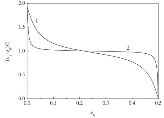
Figure 1: Dependence of the linear beam-beam tune shift on the bare tune ( $\nu_0$ ); line 1 –  $\xi = 0.05$ , line 2 –  $\xi = 0.005$ .
