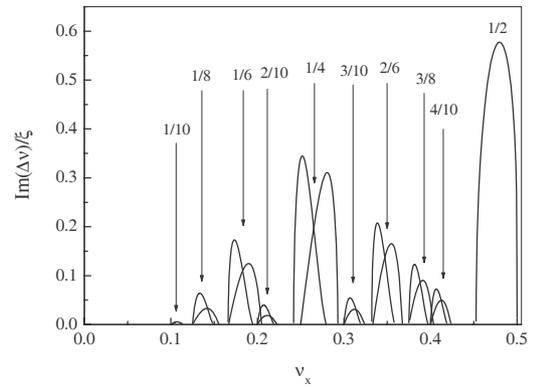
Figure 2: Dependencies of the increments of the coherent beam-beam modes on the tune of the horizontal incoherent betatron oscillations ( $\nu_x$ ). Modes  $1 \leq m \leq 5$ , arrows show positions of stopbands near particular resonances, wider curves to the right from the resonances  $\nu_x = n/(2m)$  depict the increments of the modes  $(+)$ ,  $\xi = 0.05$ .
