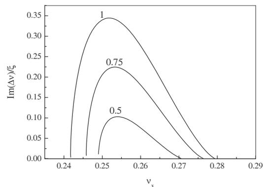
Figure 8: Modifications of the stopband of the  $(-)$  mode near  $\nu_x = 1/4$  due to hour-glass like suppression. The figures above the curves give the values of the suppression factors,  $\xi = 0.05$ .
