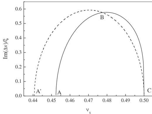
Figure 3: Dependence of the increment of the dipole mode  $(-)$  on the tune of the horizontal incoherent oscillations  $\nu_x$ . Solid line – Landau damped coherent oscillations, dashed line – monochromatic bunches,  $\xi = 0.05$ .
