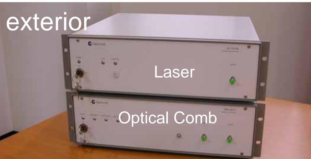
DFB Solid State Laser looked to Acetylene Absorption Spectrum (1538 nm)
