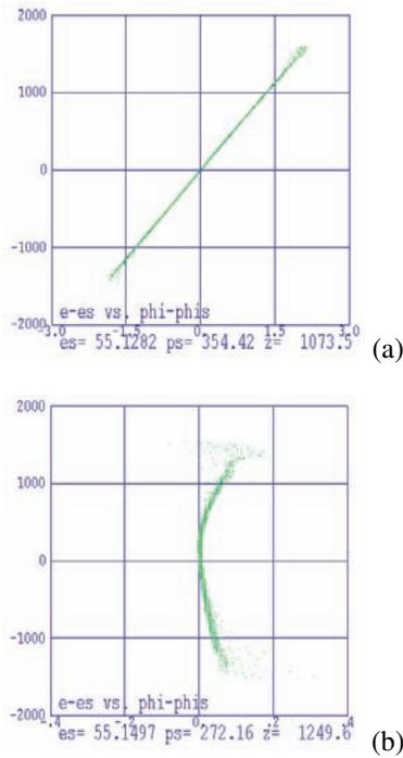
Figure 3: PARMELA simulation result: bunch shape before (a) and after (b) Chicane-2. *es* represents the synchronous particle energy, *phis* the synchronous particle phase. The vertical axis is  $e - es$  in MeV and the horizontal axis is  $\phi - \phi_s$  in degrees. One degree corresponds to about 1 ps.
