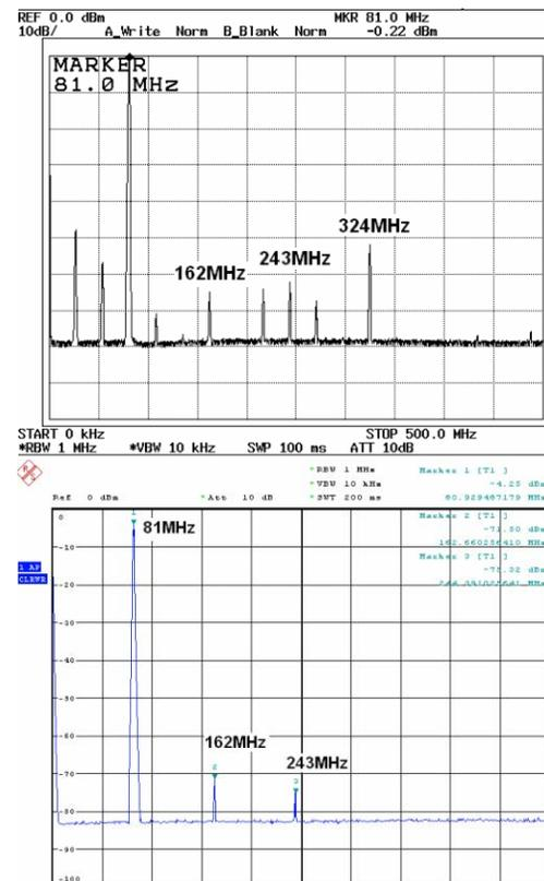
Fig. 2: Frequency spectrum of 81MHz rf signal without band-pass filter (upper) and with crystal narrow-pass filter (lower).
