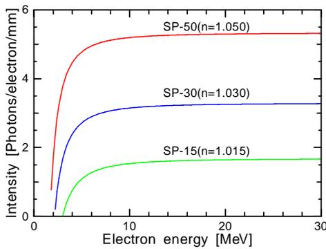
Figure 2: The number of photons as Cherenkov radiation per electron per 1 mm distance emitted from the aerogels with different indices of refraction.
