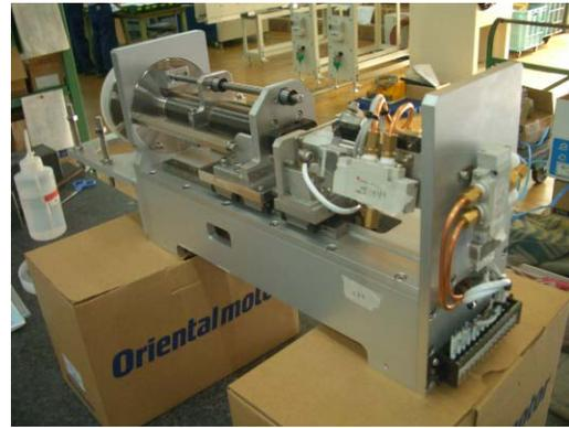
Figure 7: The drive assembly of the Cherenkov radiator with a two-staged stroke. The first stage is a profile monitor with a fluorescence ceramic screen, and the second stage is the Cherenkov radiator with the aerogel.
