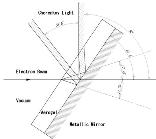
Figure 4: Schematic design of the Cherenkov radiator.
