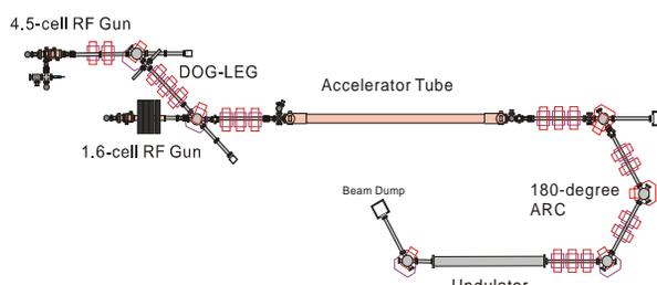
Figure 1: Schematic view of the KU-FEL driver linac.
