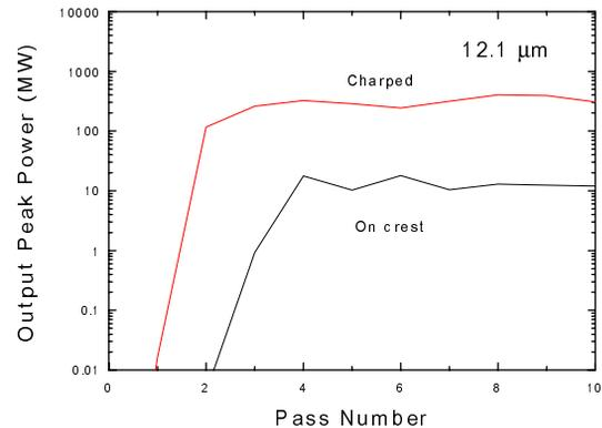
Figure 7: Round-trip development of the FEL output power.
