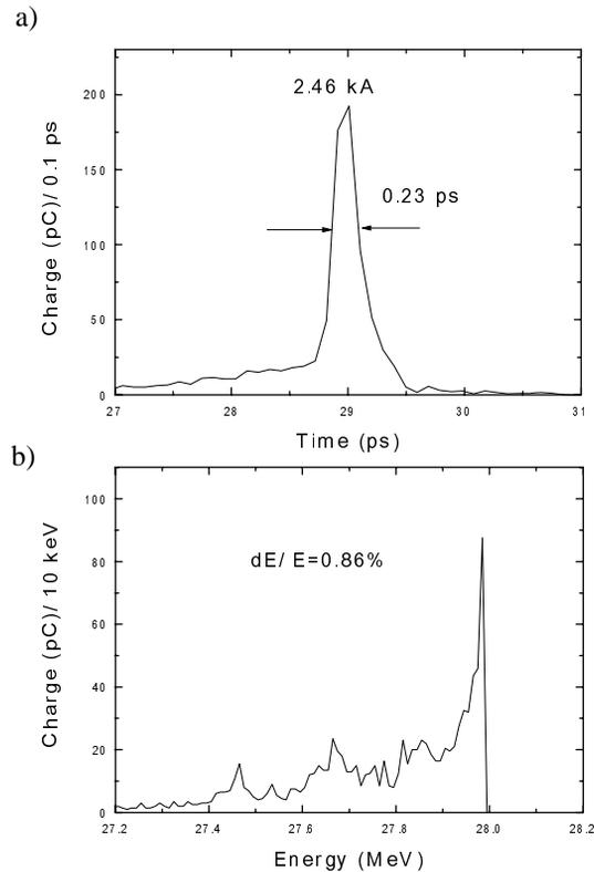
Figure 6: Time distribution (a) and energy distribution (b) at the undulator. The RF phase was ‘energy chirped mode’.
