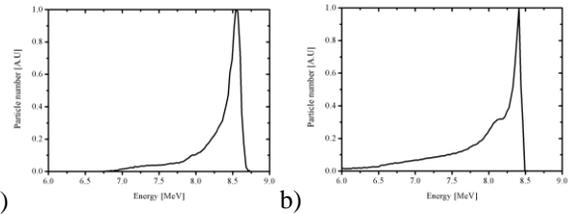
Fig. 4 Energy spread before the accelerator tube. a) Non-modulated mode b) Modulated mode
