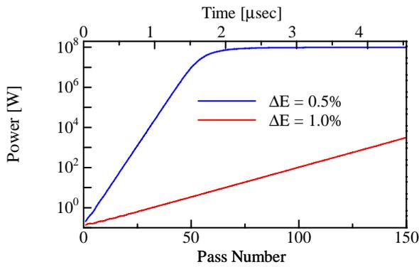
Fig. 7 FEL power evolutions for different energy spread.
