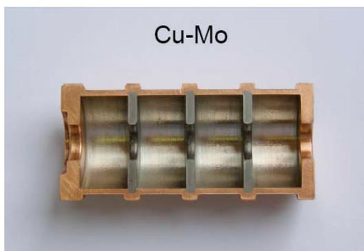
Figure 6: A Mo-Cu electroformed structure produced at INFN-LNF.
