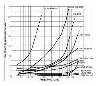
Figure 1: Illustration of penetration capabilities of different building materials as a function of frequency [4].
