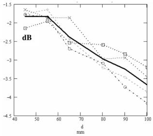
Figure 7: Measured attenuation for quasi-noise illumination in W-band as a function of sand's layer thickness for the four angular position of container: ooo - 0 deg, xxx - 90 deg,  $\Diamond \Diamond \Diamond$  - 180 deg and  $\Box \Box \Box - 270$  deg. The solid line corresponds to the averaged result.
