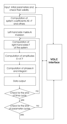
Figure 2: Block-scheme of VOLC
