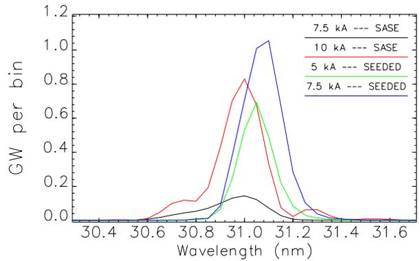
Figure 5: Predicted (GINGER calculations) output spectra at the 31-nm wavelength fundamental for the various SASE and seeded cases. Each bin is 64.6 meV wide while 1 GW is equivalent to  $1.0 \times 10^{13}$  photons.
