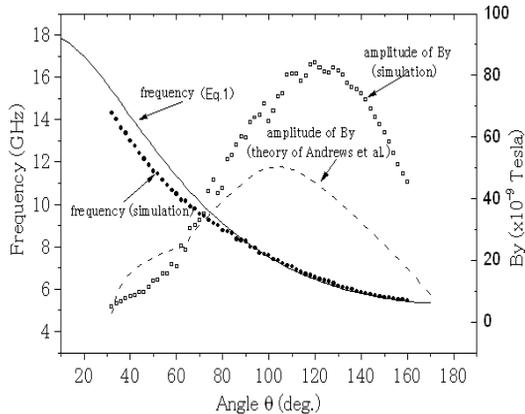
Figure 3: Distribution of SP frequency and its  $B_y$  amplitude.
