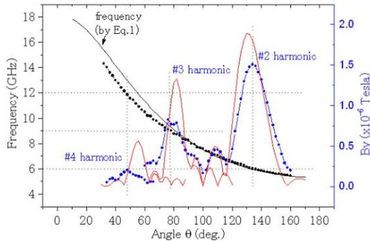
Figure 5: Distribution of superradiant SP radiation frequency and its  $B_y$  amplitude. The dotted blue line is the simulation results, and the red line the analytical result multiplied by 10.
