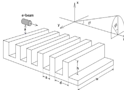
Figure 1: Three-dimensional simulation model of grating and electron beam.
